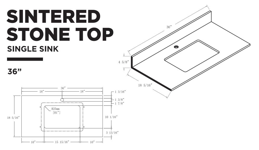
ATTENTION! Dimensions may vary by up to 3/8". It is highly recommended to pull all dimensions of actual model for installation and measuring purposes.
